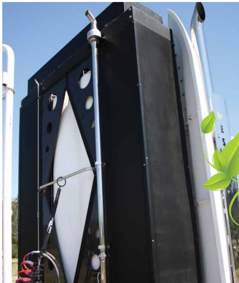
Clockwise: The CNG fuel pack contains composite carbon fibre cylinders, the four cylinders on this truck giving it a range of 800km; An alternate display shows the distance to empty and system pressure; A dash-mounted digital menu shows fuel levels and which cylinder is active
