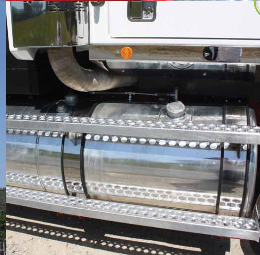
Clockwise: The hydraulic pump forces the CNG out of the fuel cylinders under high pressure; The Westport HD engine has its basis in the Cummins ISX; Simple no-fuss gas filler nozzle; The fuel tank houses both diesel and the CP-Therm hydraulic fluid in separate compartments that the system uses to inject gas into the engine
