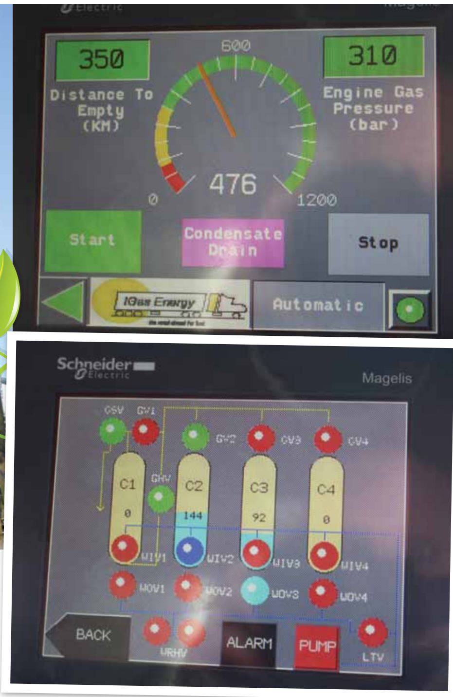
Clockwise: The CNG fuel pack contains composite carbon fibre cylinders, the four cylinders on this truck giving it a range of 800km; An alternate display shows the distance to empty and system pressure; A dash-mounted digital menu shows fuel levels and which cylinder is active
