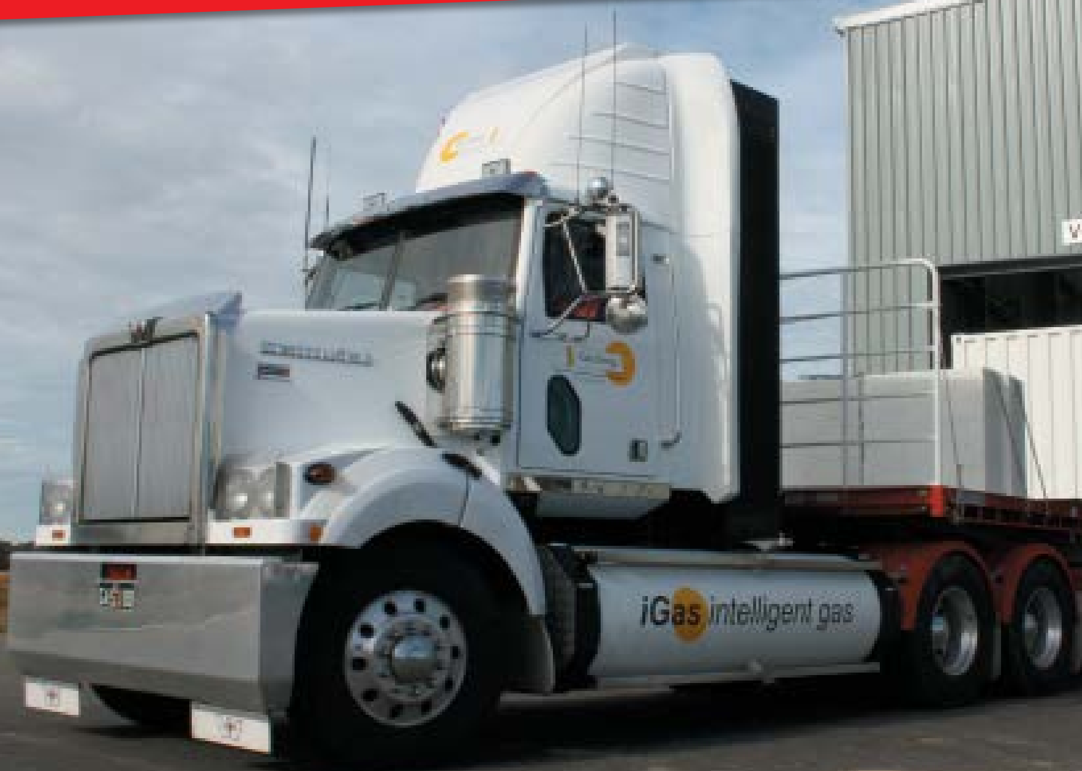
The latest incarnation of the iGas CNG adaptation; larger tanks and a new fuel delivery system have given the vehicle a longer range.
